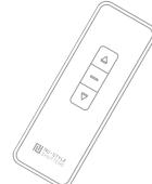
To open press up arrow button to stop press middle button & to close press down arrow button.
